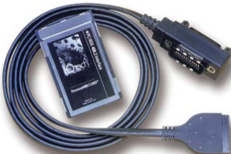
The Personal488/CARD provides an IEEE 488.2 PC-Card interface for notebook & desktop PCs
